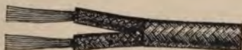
FIG. 81.—The cord of a telephone receiver. It consists of two strands of braided tinsel, insulated, and enclosed in a woven sheath. A metal pin is secured to the end of each strand, and this is inserted in the grooves of the binding-post to give electrical connection.
